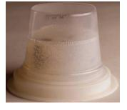
Place the mould box into the pressure pot.
