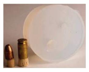
The mould is now ready for resin casting.
