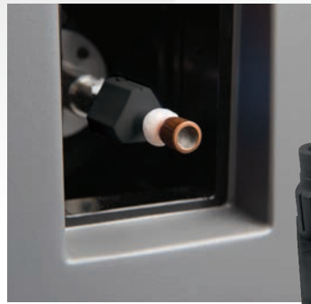
Stub is magnetically secured to shaft and automatically retracts
