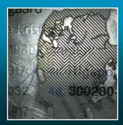
**COAXIAL LIGHTING** Coaxial or retro reflective lighting is available for examining surface structures of reflective elements.
