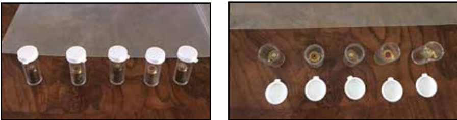
Figure 5: A flip-top vial provides easy viewing of firearm produced marks without the need to touch the cartridge case.
